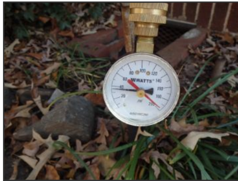
water pressure test
